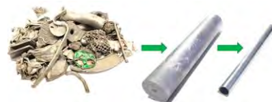
Fig. 2 Twitch scrap, homogenized billet, and extruded tube
