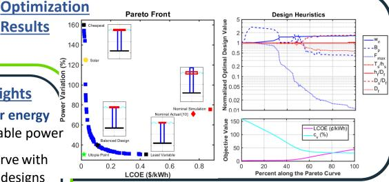
**Discussion** A tradeoff between energy cost (LCOE) and power variation (c<sub>v</sub>) suggests a possibility of a **single hardware design** across applications, with application-specific controls software.
